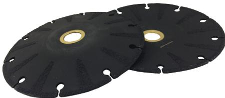
The Weha 5" Vacuum Brazed Contour Blade is designed specifically for marble and other soft stones. Perfect for cutting vanity bowls. diamonds extend a full 1 1/4" down the blade for easy bowl cutting and tight radius cuts. Very aggressive. Great life Vacuum Brazed for life and speed. 7/8-5/8 included. Part #50510
